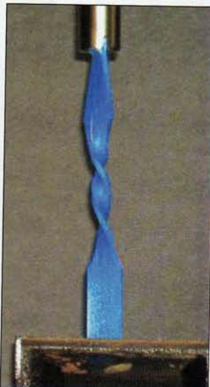
Tensile bars treated with Hybrid-Temp Rx are twisted in a torsion test. On the left is a bar produced via SLA, while the other is an SLS part. Flexibility can be improved by 300% regardless of the method used to produce the RP part, according to data published by MBD.
