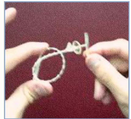
Figure 4. Enhance stresses within RP part
