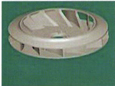
Figure 6: RP tempered SLA fan blade design.
