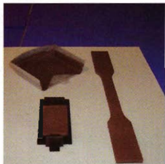
EMI and RFI shielded LS, LS, digitally printed and actual plastic parts: This picture shows a simple EMI shielding application on SL and Plastic Parts. The process is fast and easy costing 90 percent less than sending the parts out to an EMI or FRI Shielding House. This application takes only minutes to apply and can be shipped within 30 minutes. Images courtesy of Andy Pardue.
